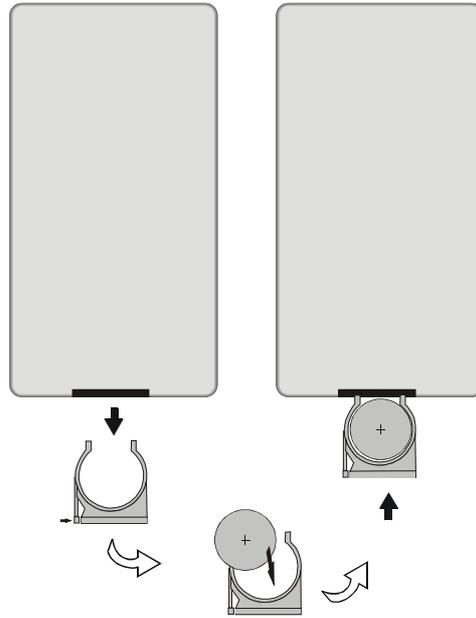
1. Refer to the drawing, take the back cover off of the remote control and remove the empty battery receptacle.
